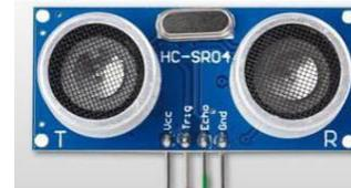
The ultrasonic sensor echo pin and trigger pin is connected to pin digital pin D7 and D8 respectively. The +VCC pin is connected to +5V supply and GND pin is connected to ground pin of Arduino Uno board. The control (PWM) pin of servo motor is connected to digital pin D9 of Arduino. Hence, servo motor is used to open the cap of dustbin. The distance can be calculated as following:  $Distance = 1/2 \times T \times C$
