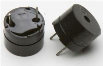
A buzzer is an audio signaling device which may be mechanical or electro-mechanical. Uses of buzzer is to indicate the bin is full. We have given 5v supply to buzzer.
